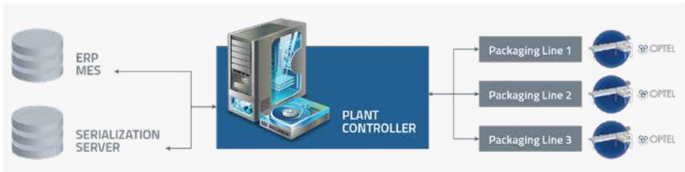
Figure 4. Plant controller and its relation to other elements.
